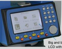
Big and backlighted LCD with indications of electronic level
